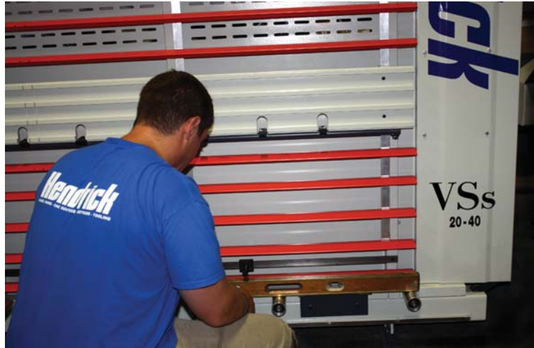
Monthly inspection of material support rollers for Hendrick VSs Vertical Panel Saw.
