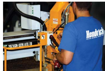
Semi-annual router spindle lubrication on Hendrick 20ZXGN CNC Router.
