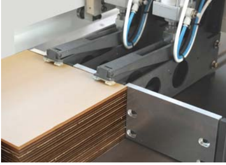
Unique solid pusher/gripper combination is ideal for cutting small parts, rod and tubing.
