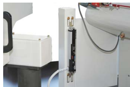
Full-length electronic light curtain provides enhanced safety within the cutting area.
